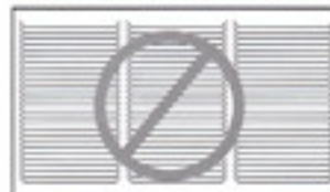
INCORRECT Horizontal Louvers
